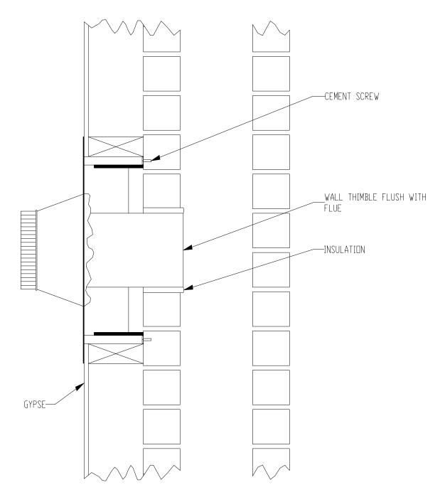
FIGURE 2.2.2 (B) Factory Built Thimble
